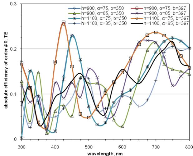
Figure 7. Efficiency of  $0^{\text{th}}$  order of a Si trapezoidal grating, with different profile parameters and  $\theta = 40^\circ$ , plotted vs  $\lambda$ .
