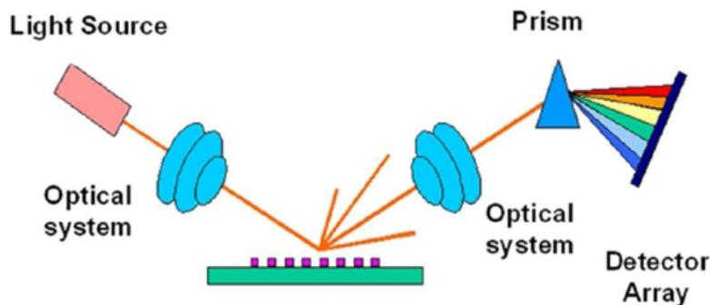
Figure 1. Schematic of a spectroscopic scatterometry setup.
