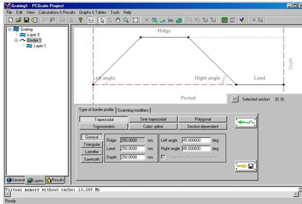
Figure 2. General trapezoidal profile obtained by cutting the surface of a grating with one vertical plane.
