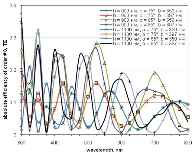
Figure 6. Efficiency of  $0^{\text{th}}$  order of a Si trapezoidal grating, with different profile parameters and  $\theta = 0$ , plotted vs  $\lambda$ .
