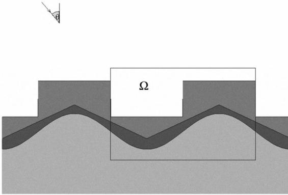
Figure 3: Schematic cross section of a grating with penetrating boundaries.
