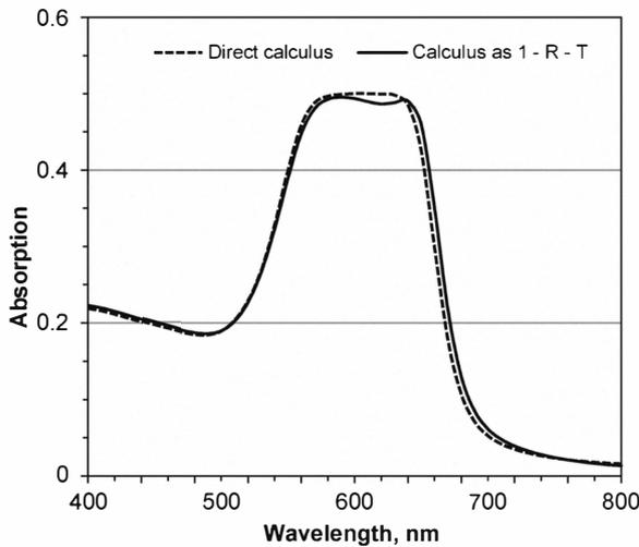
Figure 4: Absorption of a grating with Au rectangular nanorods embedded in a dielectric medium vs wavelength.
