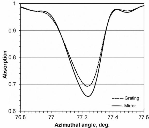
Figure 5: Absorption of W/B<sub>4</sub>C multilayer structures working in a conical mount vs incidence angle of x-ray radiation.
